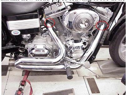
4) Slip on new muffler over collector leaving loose, turn muffler to put bolts at 8 o' clock.
