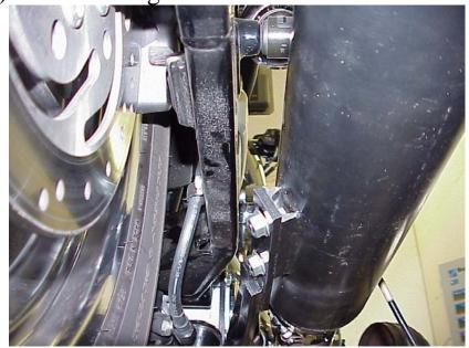
7) Tighten Up all other bolts in order back to front. Not forgetting to tighten up the foot peg.
