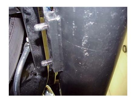
5) slide new bracket onto bolts hand tighten.
