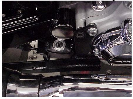
6) Install and tighten nuts to bottom of muffler.
