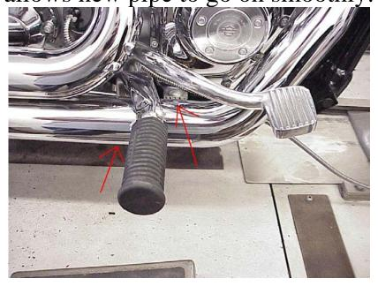
3) Install new head pipes leaving loose at head.
